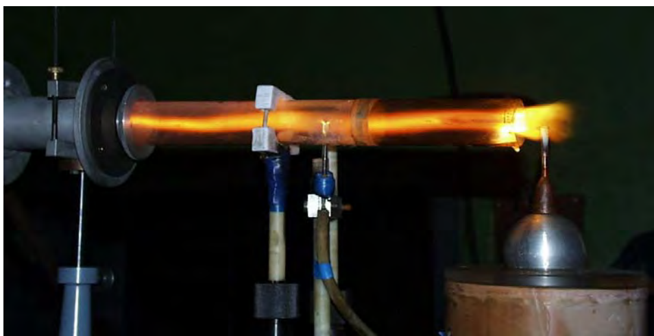
Fig.1.14. Internal PAC. Red flame. HF discharge. M=1,2 ; P_{st}\sim 1 Bar, fuel-airflow equivalence ratio \phi=0,7 ; CH 2 radical generation
