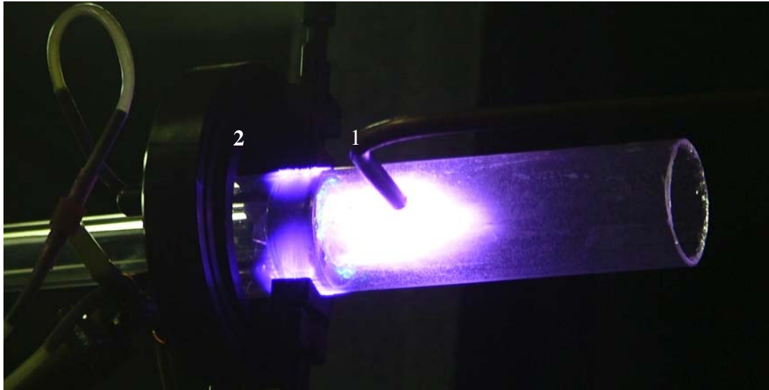
Fig.1.4. HF discharge in supersonic airflow ( M=1,2 ; P_{st}\sim 1 Bar, T^*=297K ). 1- “hot” HF electrode, 2- grounded step-electrode (propane is injected through this electrode)
