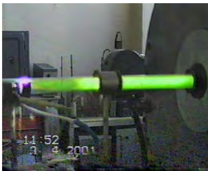
Fig.1.15. Internal PAC. Green flame. Combined discharge. M\sim,2 ; P_{st}\sim 200 Torr, fuel-airflow equivalence ratio \phi=1,1 ; C 2 radical generation
